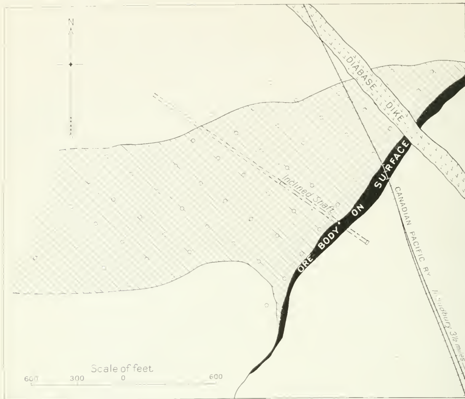
Fig. 51—Map showing Murray ore body, Sudbury area, Ontario. The shaded area denotes the known extent of the deposit below the surface; the ore body dips to the northwest at an angle of 36° as shown in Fig. 52. The small circles indicate diamond drill holes. From drawing by the British America Nickel Corporation.
